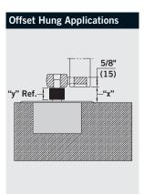
Extended Spindle Insert NOTE: Closer and arm must be installed per template for door clearances shown to be valid.
