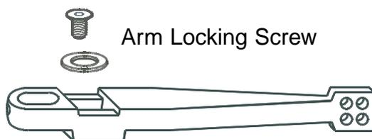
For center hung applications, the door must be removed to access the arm locking screw. Once the door has been removed, tighten the screw securely down through the washer and onto the closer spindle. Once door is rehung, install/tighten arm alignment screws and washers.
